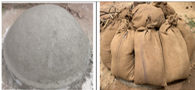
Figure 6. EPSC spherical shell a) freshly casted b) loaded with uniform pressure
